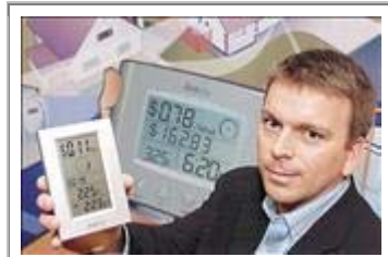
Danny Tuff, president of Blue Line Innovations Inc., displays a PowerCost Monitor, a wireless device that reads electrical meters and translates that information into megawatt hours of electricity. The device allows homeowners to tell how much electricity they're using and how much it costs. (Photo: By JOE GIBBONS/The Telegram)
